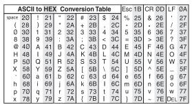
Figure 19. ASCII to Hexadecimal Conversion
